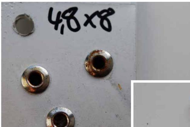
Following pictures show CUP sealed blind rivets of stainless steel A2 (AISI 304 / 1.4301) with a martensitic mandrel of stainless steel (AISI 410 / 1.4006 or AISI 420 / 1.4021), which were subjected to a Kesternichtest (DIN 50018 2.0s / DIN EN ISO 6988). Samples of our competitors as well as our own were tested.
